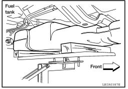
Remove the fuel tank straps and slowly lower the fuel tank to access the top of the fuel level sensor, fuel filter and fuel pump assembly.
