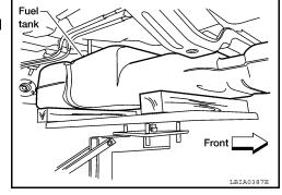
9. Remove the fuel tank straps and slowly lower the fuel tank to access the top of the fuel level sensor, fuel filter and fuel pump assembly.
